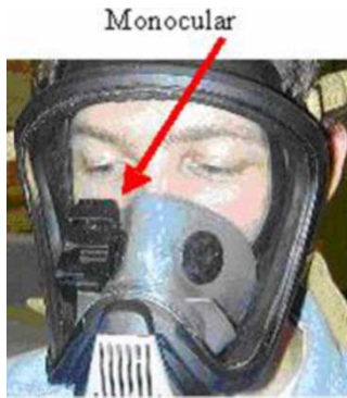
Fig. 1 Prototype fire-fighter monocular HMD in facemask
