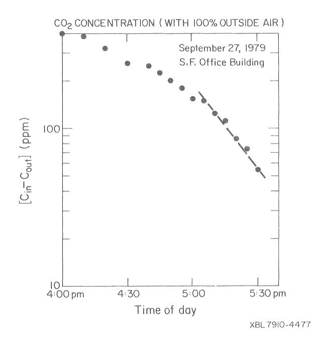
Figure 4 Carbon dioxide decay curve for the all-outside-air mode.
