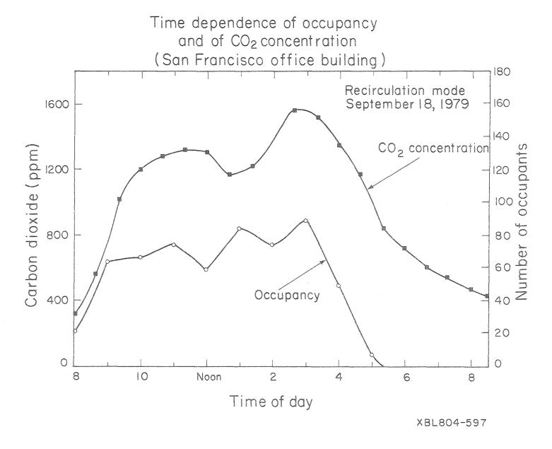
Figure 2 Time dependence of occupancy and of carbon dioxide concentration in the waiting room of the San Francisco Social Services Building. The ventilation system is in the recirculation mode.
