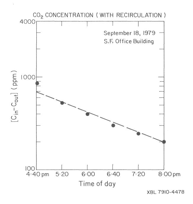
Figure 3 Carbon dioxide decay curve for the recirculation mode.
