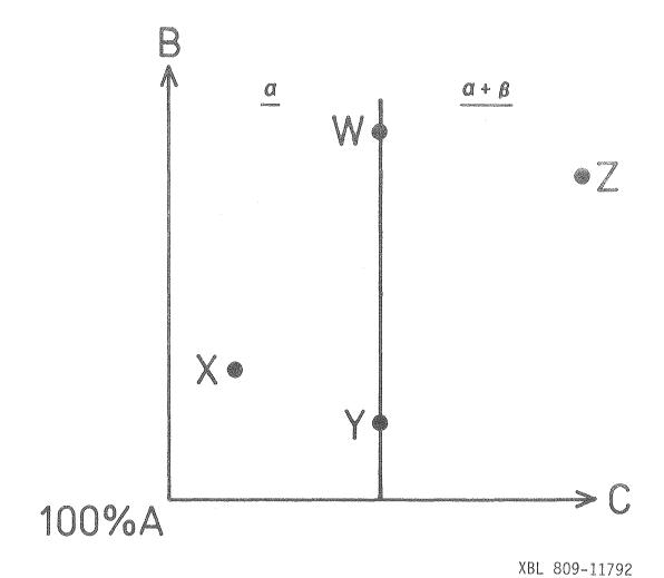
Figure 2. Isothermal Section of ABC Phase Diagram.
