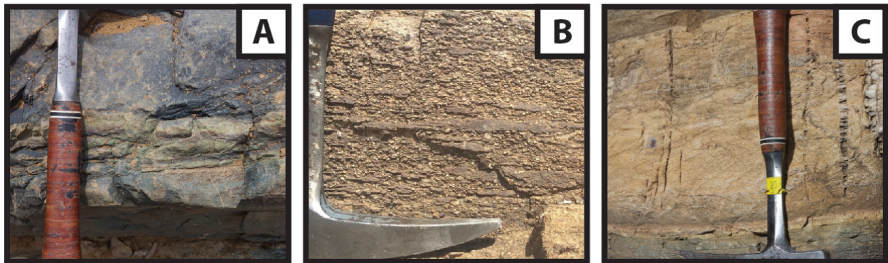
Figure B.2: (A) Photograph of the lava flow T1b-439.8Z. (B) Photograph of the ignimbrite T39-108.0Z, with feldspar phenocrysts and fiammed lithic clasts. (C) Photograph of the 30 cm rhyolitic tuff T39-420.2Z, with normally graded lapilli at the base. Hammer points up section in all panels.
