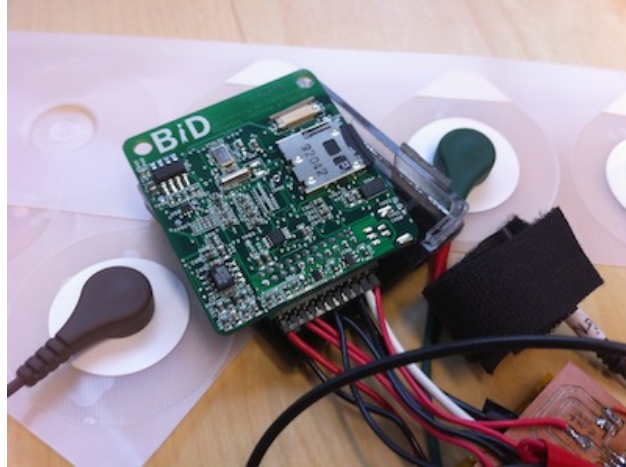
Figure 6.3: Wireless monitor with sensors
