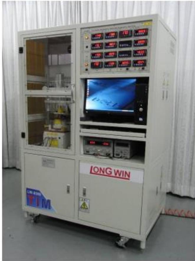
**Figure 3.1:** TIM tester (LonGwin) used to conduct all thermal measurements for noncuring thermal interface materials used. This instrument allows for various aspects to be controlled while measuring including pressure, temperature control of measurements. Nanofabrication Facility, UC Riverside, 2019.
