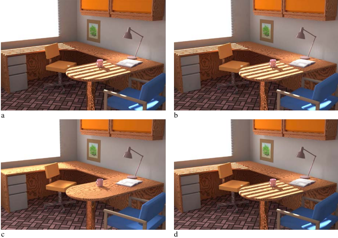
Fig. 2. Office with Venetian blinds showing a) standard backwards ray-traced rendering without mkillum or BSDF data (some sampling artifacts are visible on the wall near the desk), b) mkillum 1- without BSDF data (note smoother shading on wall near desk), c) mkillum 1+ where window is a standard light source with a computed candlepower distribution (the average behavior is correct but appearance of blind and shadows are lost), and d) mkillum 1- with BSDF data and blind geometry allows direct beam penetration with shadows from the blind slats.
