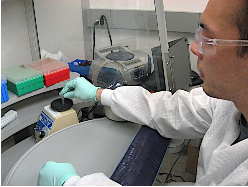
Figure 13. Final Design of Biosafety Cabinet Design. Design includes sunken area for commonly used equipment to reduced shoulder postures and improved work efficiency.
