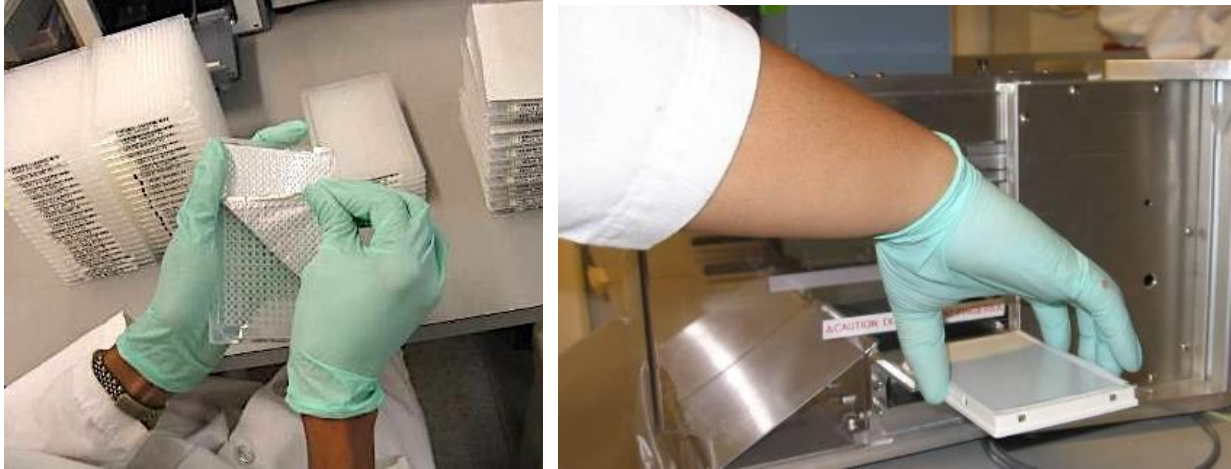
Figure 16 (left). Before. Pulling the aluminum seal off a 96-well plate requires near maximum hand strength and was identified by employees as one of the most physically demanding tasks. Figure 17 (right). After. A custom machine was designed and built to mechanically remove the seal. Loading the plates is quick and easy.
