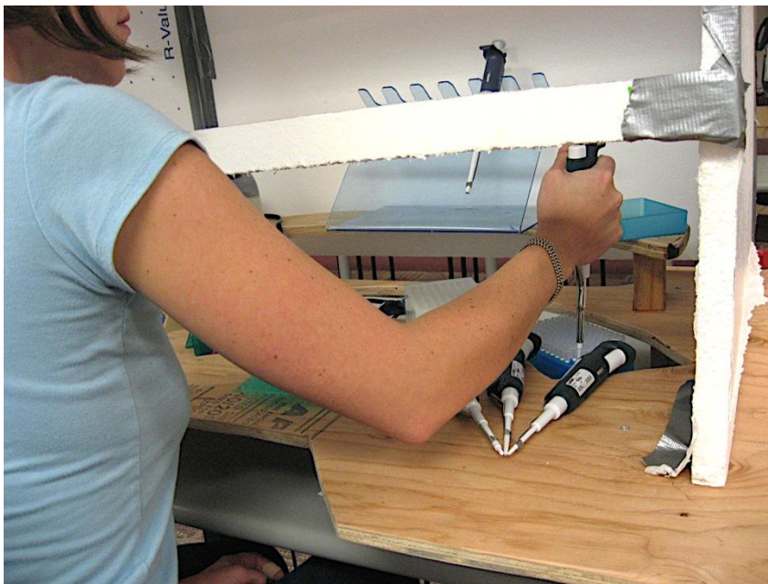
Figure 12. Participatory Design Process. Usability testing of a prototype biosafety cabinet.
