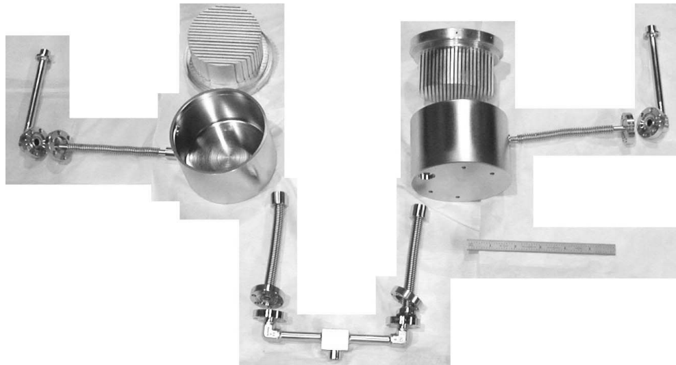
FIGURE 4. Parts of the helium condenser and piping before assembly
