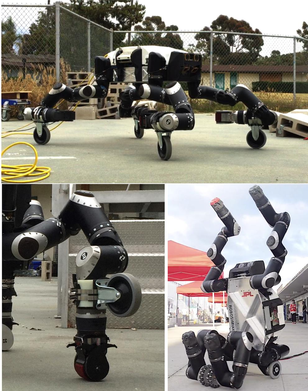
Figure 2.3: RoboSimian on wheels.
