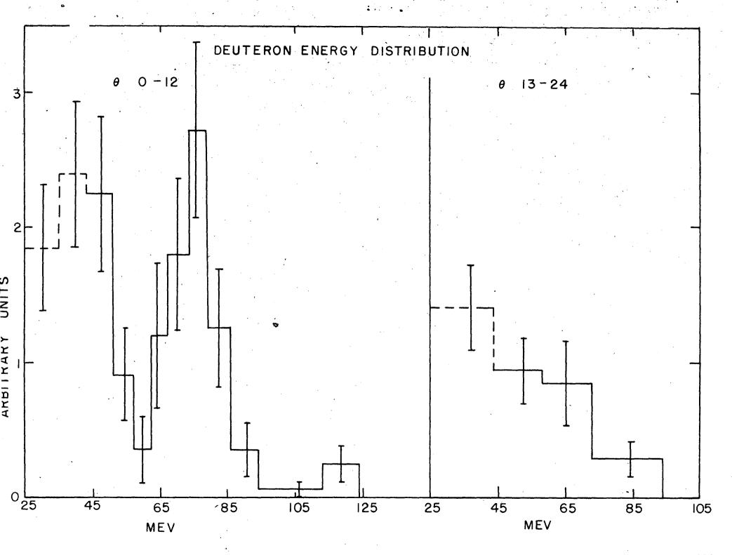
Figure 2a - Energy distribution of the protons leaving carbon within 12° of the neutron beam.
