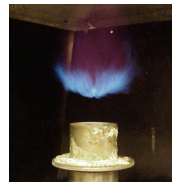
Figure 4. A 12.7-cm UCLSB designed for water and steam boilers. The flame is highly lifted to optimize performance in boiler tubes.
