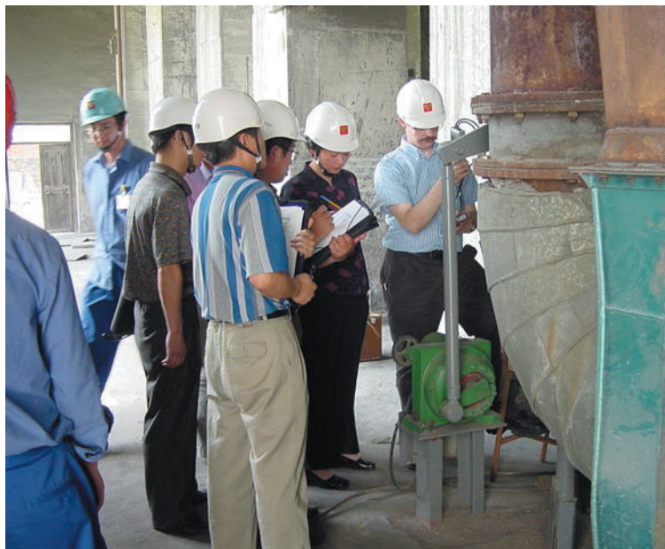
Figure 1. Fan expert Ron Wroblewski (right) demonstrates how to conduct fan flow measurements.
