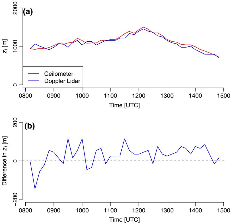
**Fig. 7** Time series of ABL heights retrieved from side-by-side measurements of a ceilometer and a Doppler lidar (a) and the difference between the instruments (b)
