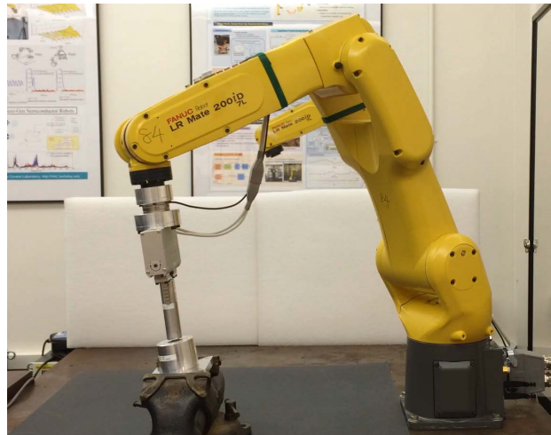
Figure 3.8: Peg-hole-insertion testbed. The diameters of peg and hole are 25.370mm and 25.400mm respectively, with 0.030mm clearance (H7h7 tolerance). The model of industrial robot is FANUC LR Mate-200iD.
