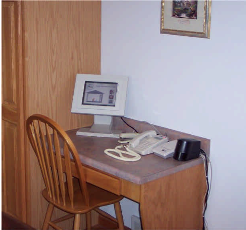
Installed Whirlpool energy monitor touch-screen
