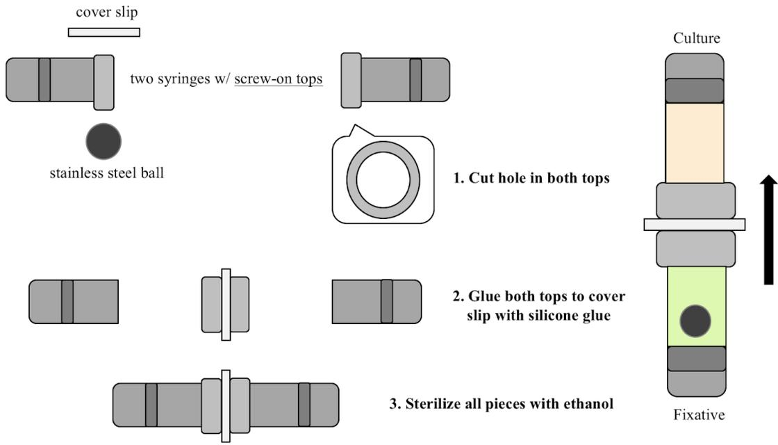
**Figure 2. Diagram of *in situ* fixation under high hydrostatic pressure.** The black arrow indicates the direction the incubation device should be placed under high pressure to prevent the stainless-steel ball from breaking the coverslip prematurely.
