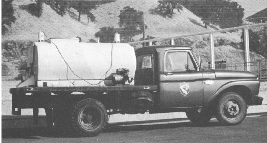
FIGURE 73—A 400 gallon fish planting tank is mounted on a flatbed pickup truck. It is equipped with a small electric pump at each end of the tank which operates from a generator or a heavy duty truck battery and sprays the water to the middle of the tank. It holds the temperature very constant. Photograph by George Bruley, 1973.
