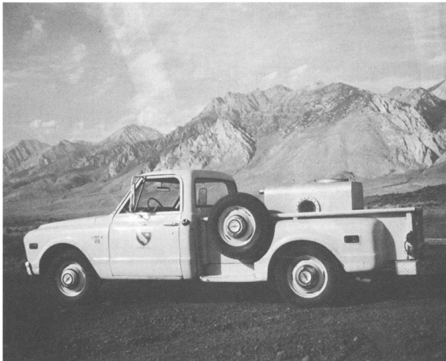
FIGURE 74—Several 150 gallon fish planting tanks are mounted on pickup trucks. The pumps are gasoline driven. Ice is used for refrigeration. Photograph by George Bruley, 1973.
