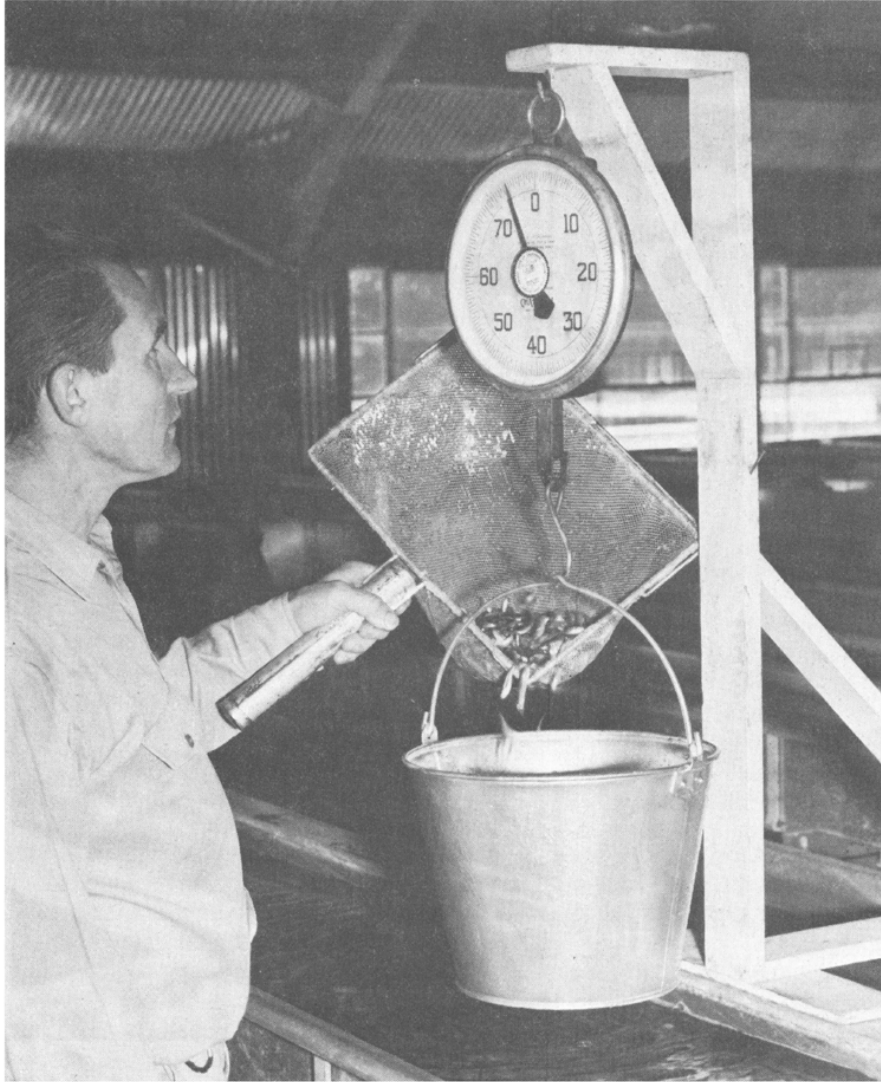
FIGURE 68 —Spring balance scale suspended over hatchery trough for weighing fingerlings. Photograph by J.H. Wales, 1959.
