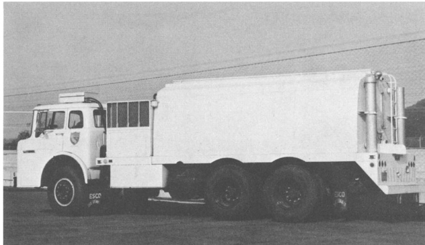
FIGURE 70—A 2500 gallon fish transport truck. The water pumps and refrigeration units are operated by electricity which is generated by a diesel driven unit on the truck. Photograph by George Bruley, 1973.
