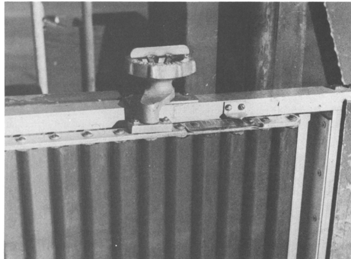
FIGURE 65—Wilco adjustable grader. A , grader bars are in the open position which can be adjusted by turning the knob on top of the grader and locking it with the thumb nut; B , grader bars are closed; note the position of the knob on top of the grader; graders can be made any length required. Photographs by George Bruley, 1973.
