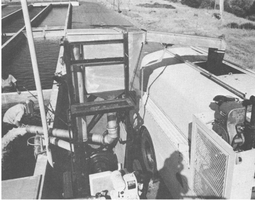
FIGURE 67—Fish pump loading a tank truck. Fish are sucked out of the pond, pass through the pump, pushed up to the separator tower and spilled onto a grader rack which slopes downward. The large fish slide across the grader rack and go into the tank truck. The small fish and water drop through the rack and return to a pond via a hose. Photograph by George Bruley, 1973.
