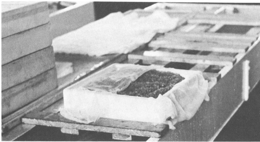
FIGURE 43—A, lightweight egg shipping case; and B, tray packed with eggs which is placed in the cardboard carton inside a leak proof plastic liner. Photographs by Jerry Eskew, 1973.
