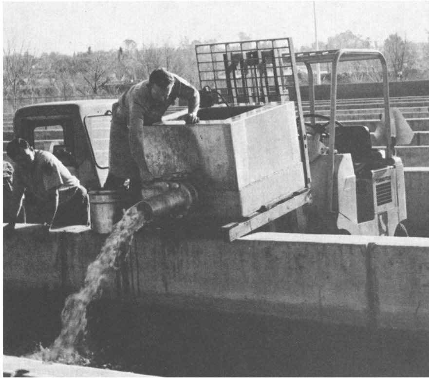
FIGURE 75 —This small 100 gallon utility tank is used on the hatchery grounds to move fish. It can be moved about with a fork lift. Photograph by George Bruley, 1973.
