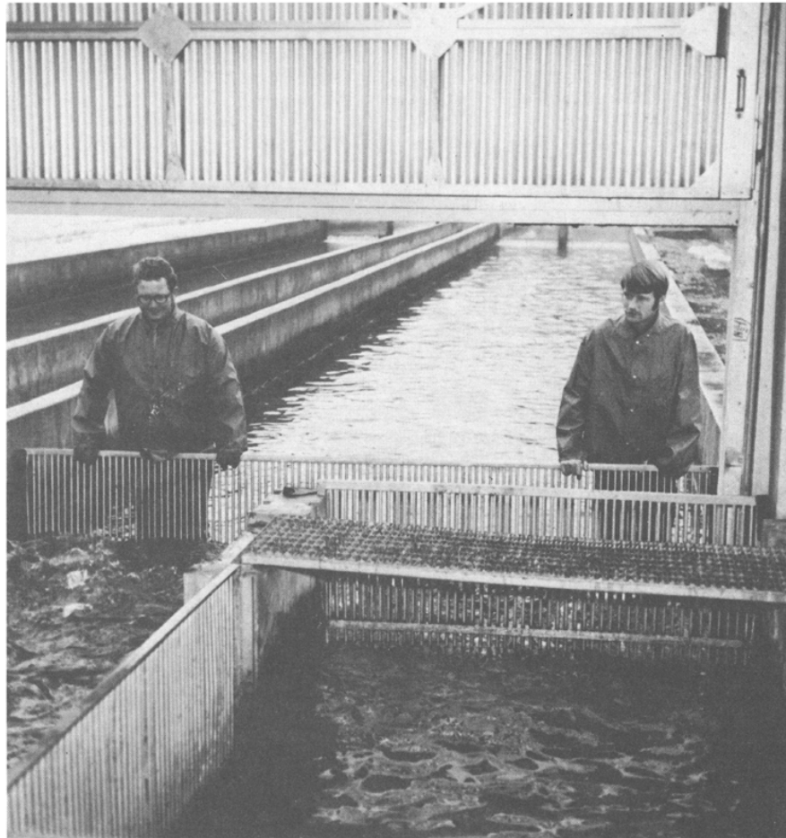
FIGURE 11—Brood fish being moved into the spawning house for sorting and spawning. Note the overhead door that can be lowered into the water to keep the spawning house warm during winter months (also shown in Figure 9). Pens can be made with crowding racks for use during the sorting and spawning operations. Photograph by George Bruley, 1973.
