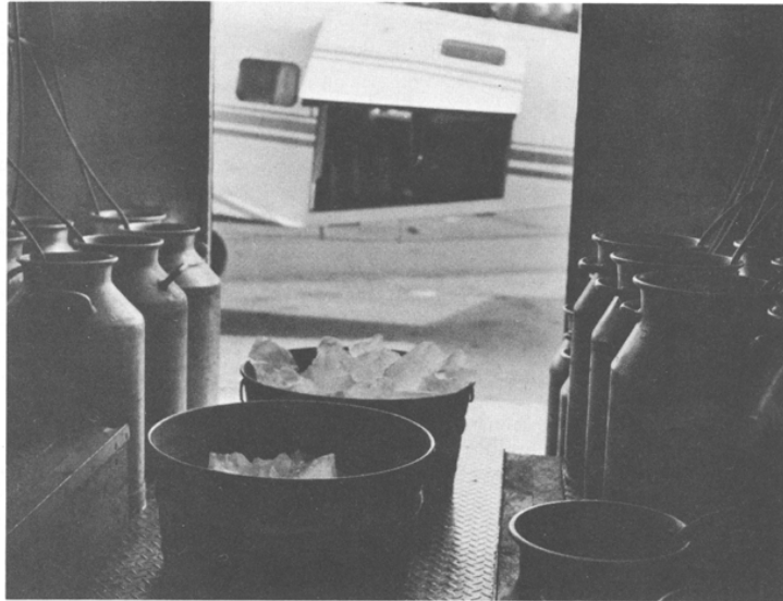
FIGURE 77—A, refrigerated van truck is desirable to haul cans of fish to the airplane because the temperature remains more nearly constant; B, hoses can be seen which supply air to the cans from air compressors driven by gasoline engines. Photographs A by T. T. Jackson and B by George Bruley, 1973.
