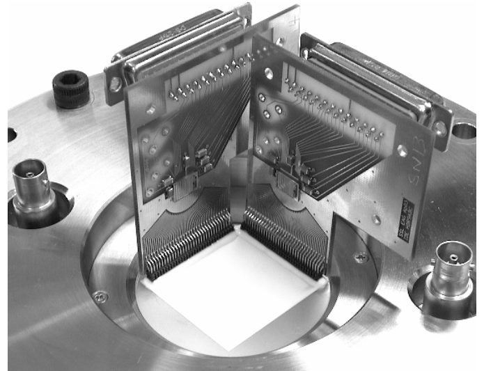
Fig. 2. A photograph of back end of the XS anode with the two ASIC chip carrier boards plugged into the back-end connectors.
