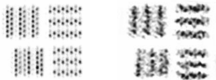
Fig. 8. Zoomed images of Group 5 elements 5 and 6 of the resolution mask. (left) a negative optical microscope image; (right) UV image obtained with the XS detector.
