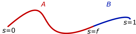
Figure 1.1: A schematic of an AB diblock copolymer chain indicating contour positions s = 0 , f , and 1.
