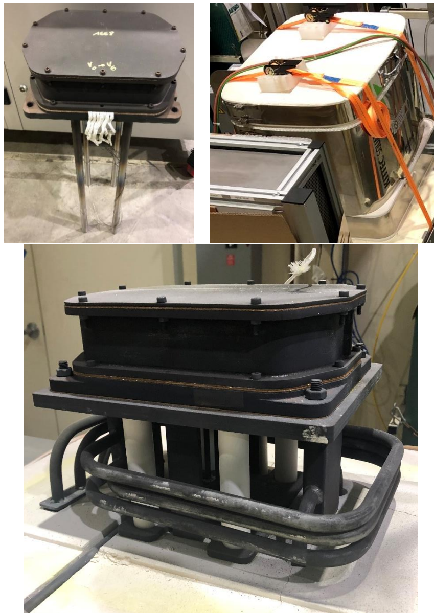
Figure 69: 6-cell short stack and electric furnace to thermally manage the short stack.
