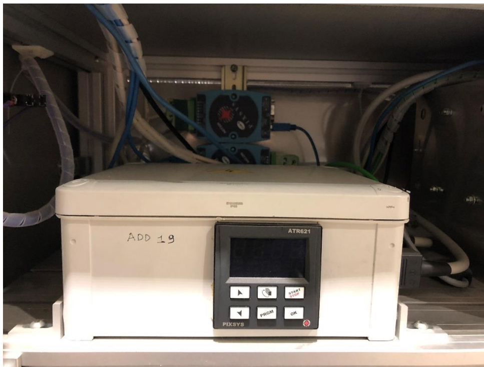
Figure 70: Independent temperature controller (PIXSYS ATR621) to control furnace temperature.
