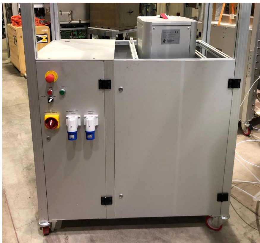
Figure 75: Evaporator and reformer reactor.
