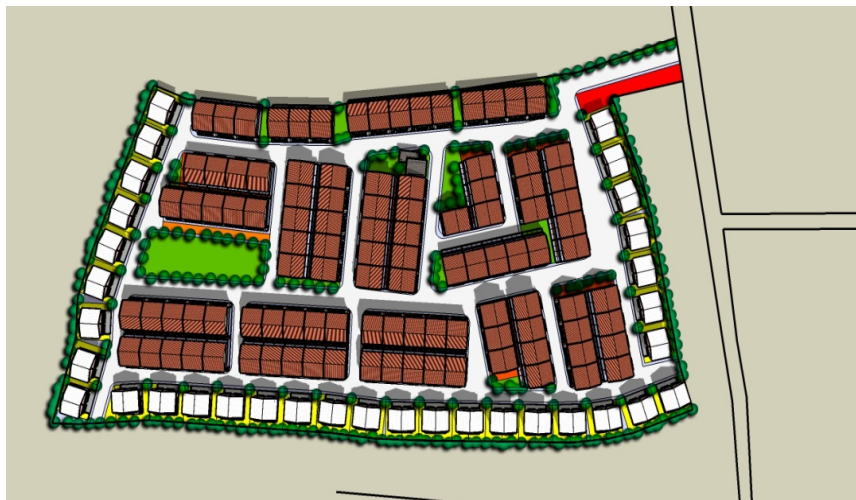
Figure 4.2: CODI Community Plan. Note the single point of entry and exit as well as common green space. Source: CODI
