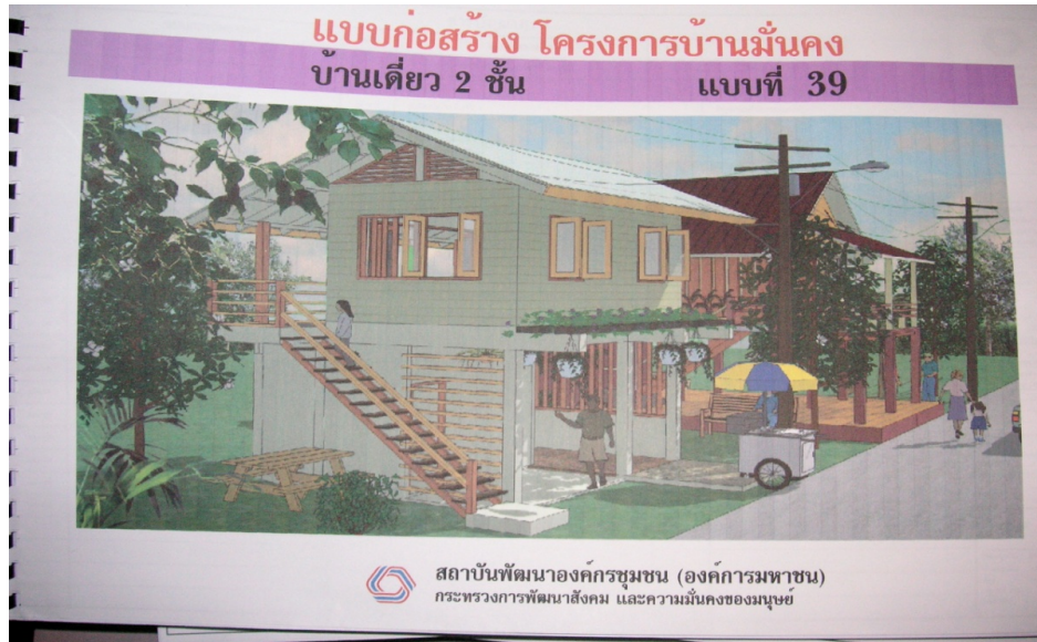
Figure 7.7: CODI home design. Note vernacular features like, passive cooling vents in the roof and the traditional raised post construction. Source: N/A
