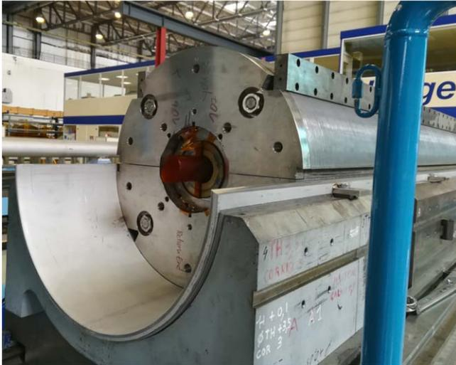
**Figure 18.** Collared coil enclosed in the laminated yoke before shell welding.
