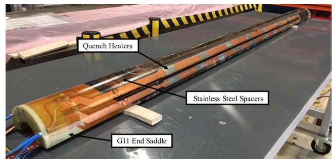
**Figure 7.** View of an 11 T coil after impregnation.
