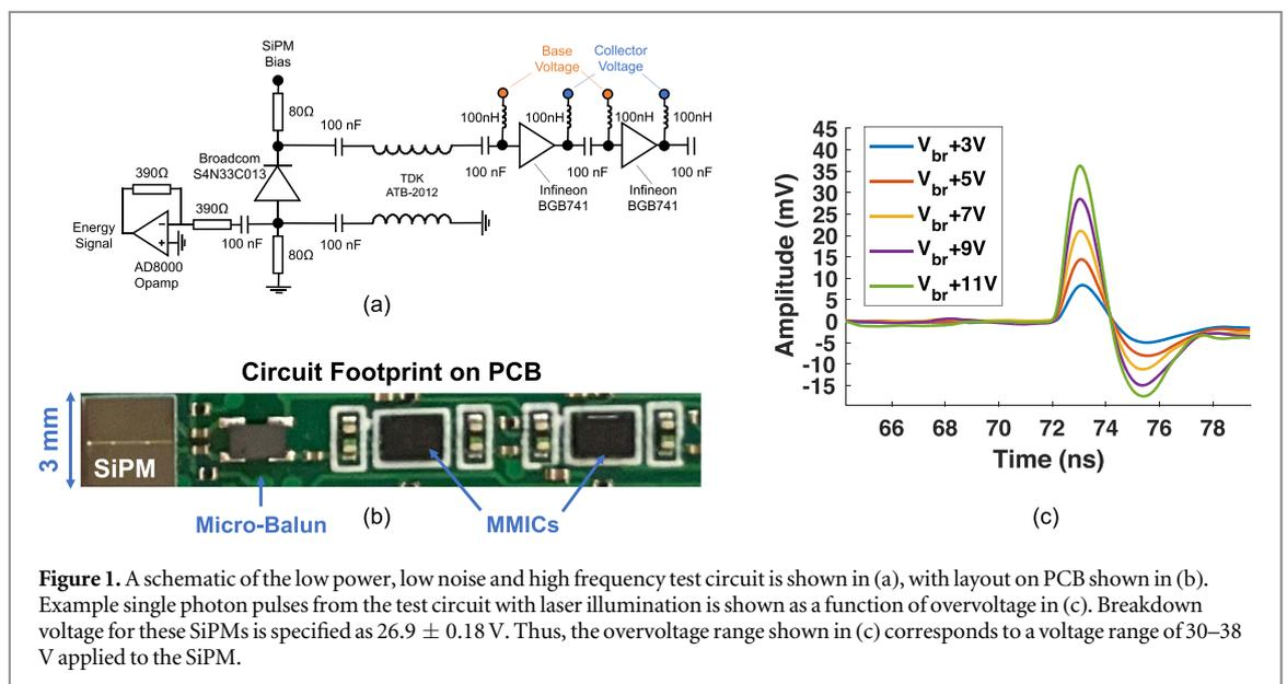
**Figure 1.** A schematic of the low power, low noise and high frequency test circuit is shown in (a), with layout on PCB shown in (b). Example single photon pulses from the test circuit with laser illumination is shown as a function of overvoltage in (c). Breakdown voltage for these SiPMs is specified as  $26.9 \pm 0.18$  V. Thus, the overvoltage range shown in (c) corresponds to a voltage range of 30–38 V applied to the SiPM.
