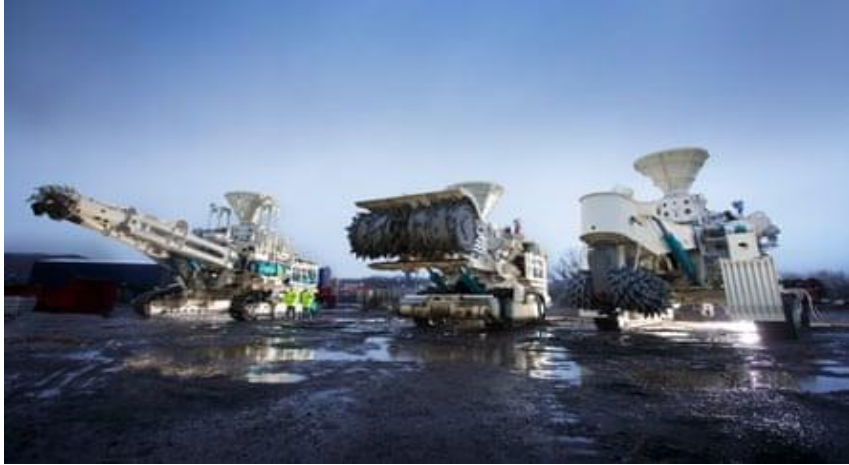
Figure 4.2: Underwater mining vehicles used off the PNG coast for taking rock samples. Photograph: Nautilus minerals.
