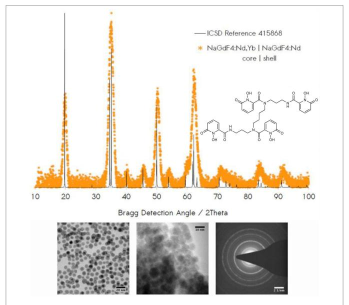
FIGURE 1 | Top: Powder XRD data confirm colloidal synthesis of the hexagonal NaGdF<sub>4</sub>:Nd, Yb | NaGdF<sub>4</sub>:Nd. Inset: **343** surface chelator. Bottom: TEM reveals monodisperse nanocrystals of 10 nm in diameter in cases of unmodified (left) and **343**-chelated (center) samples. Electron diffraction (right) provides evidence of dominant Bragg diffraction from lattice planes of hkl indices: (100), (110) + (101), (201), and (300) + (121).
