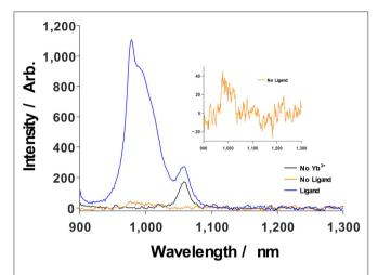
**FIGURE 3** | Ligand sensitization significantly enhances Yb<sup>3+</sup> luminescence upon excitation at 350 nm (blue), relative to the case of NP illumination in the absence of photosensitization by **343** (orange, inset). Sensitized NPs without Yb<sup>3+</sup> only show Nd<sup>3+</sup> emission at 1057 nm (black).
