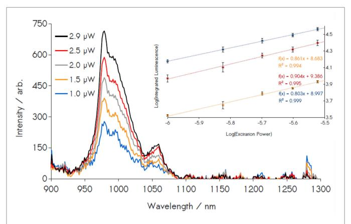
**FIGURE 5** Power dependence study of 3/20% doped Nd<sup>3+</sup>/Yb<sup>3+</sup> NPs. Emission spectra are integrated in the region of Yb<sup>3+</sup> luminescence (940–1040 nm) and plotted against the excitation power (inset). The power dependence of these material exhibits a sub-linear slope, with a total of 10 independent measurements yielding an average slope of 0.86 ± 0.04 among three replicates, confirming the presence of two-photon emissions.
