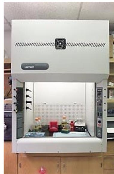
**Figure ES-5. Labconco alpha prototype Berkeley Hood.**
