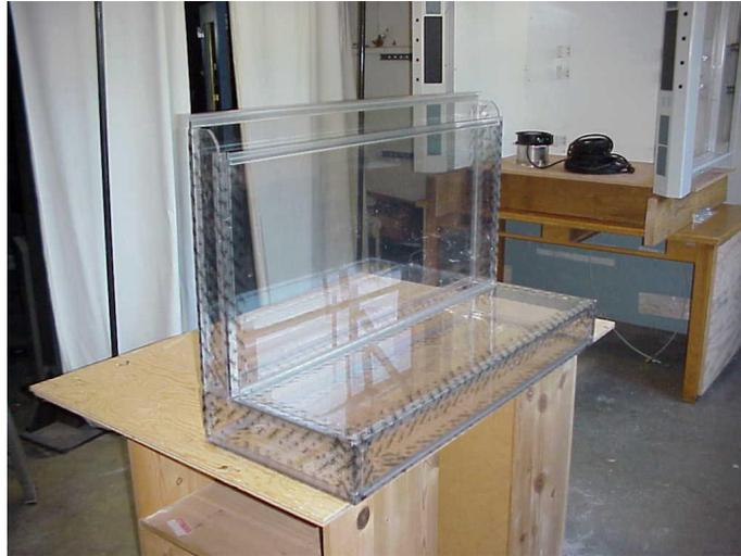
**Figure 5. Clear plastic plenum to facilitate visual tests**
