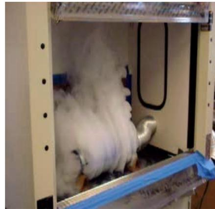
**Figure 11. Berkeley Hood, showing full containment.**
