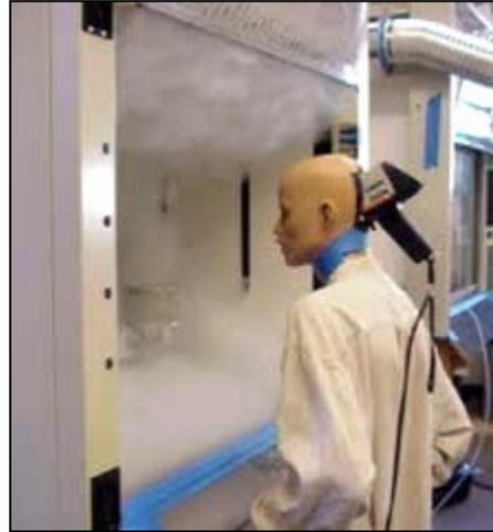
**Figure 10. Berkeley Hood, showing patented air-divider supply effect.**
