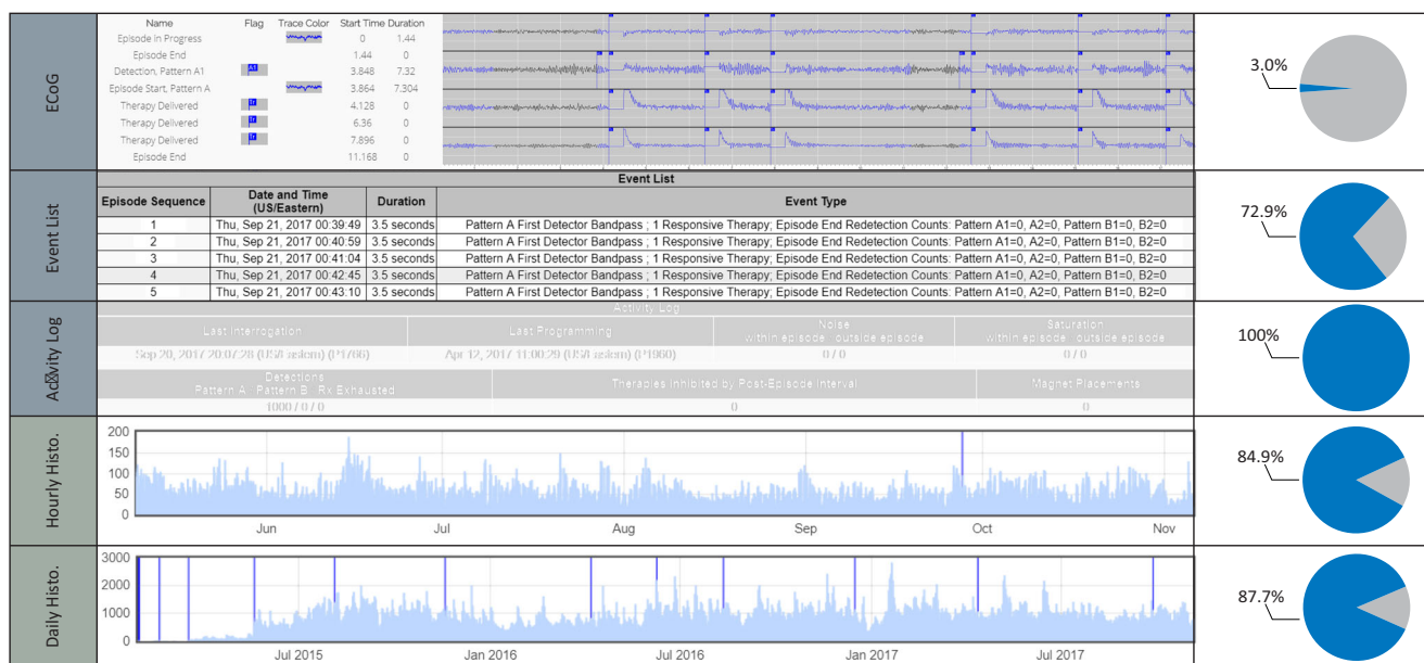
Fig. 2 Levels of RNS System detailed and summary logging. Completeness of each source of logging information relative to the Activity Log, which is the most complete but least detailed logging source, is shown in pie charts. Representative screen captures of the NeuroPace PDMS provide a basic reference of the primary sources of
