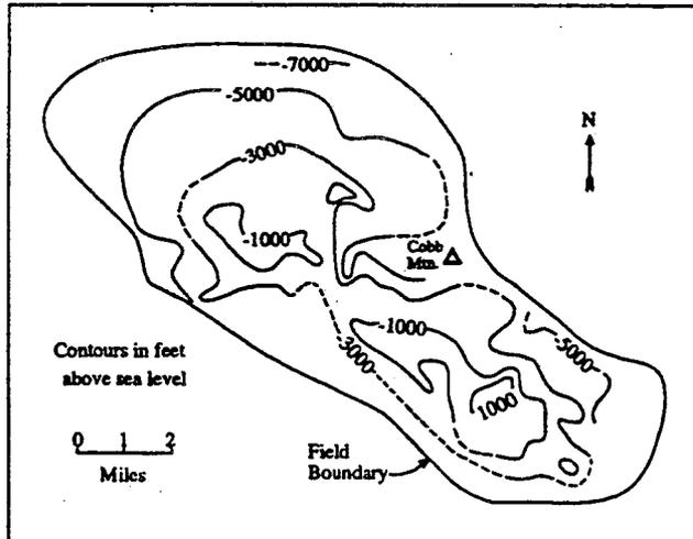
Figure 5. Elevation of the top (first steam entries) of The Geysers reservoir (after Field Operators, 1992).
