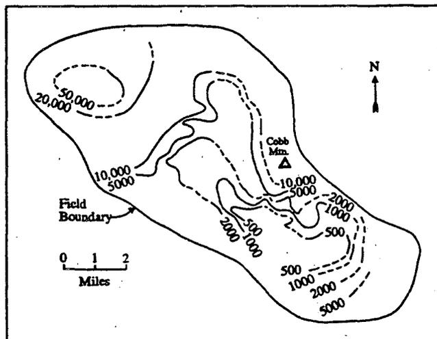
Figure 1. Initial (early-production) distribution of noncondensable gas in steam from The Geysers reservoir (in parts per million by weight) after Gunderson (1989) with some additional estimated contours.
