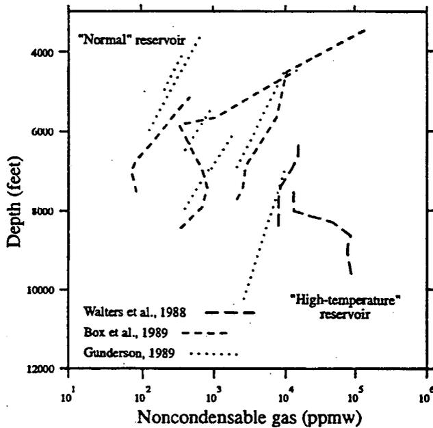
Figure 3. Variations with depth of gas concentrations (in parts per million by weight) in steam from The Geysers "normal" and "high-temperature" reservoirs.
