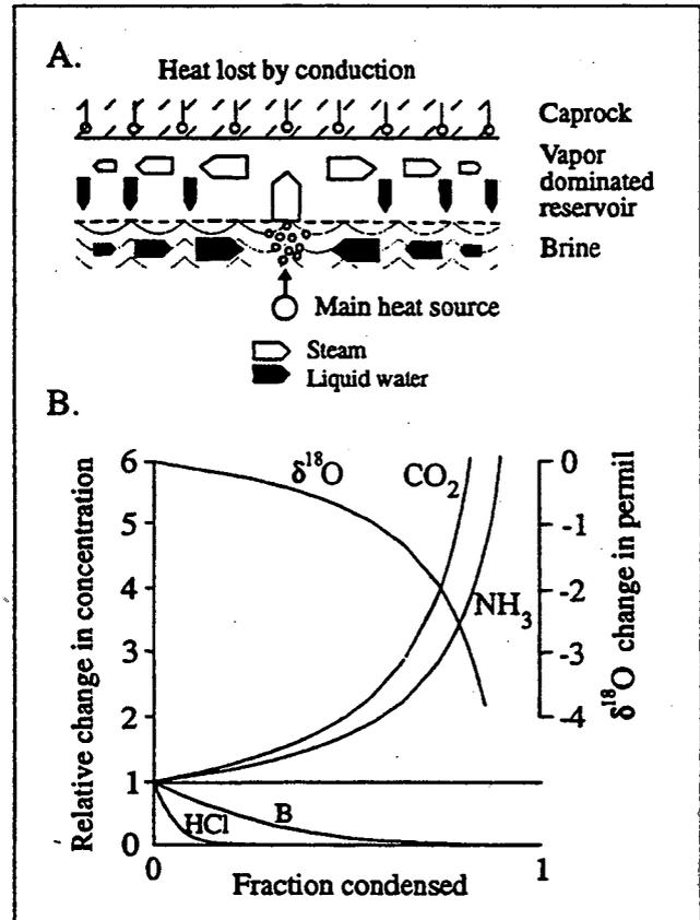
Figure 4. (A) Schematic fluid flow, boiling and condensation in a vapor-dominated geothermal reservoir and (B) effects on gas concentrations and  $\delta^{18}\text{O}$  values in steam due to partial condensation in a Rayleigh process during lateral flow (after D'Amore and Truesdell, 1979).
