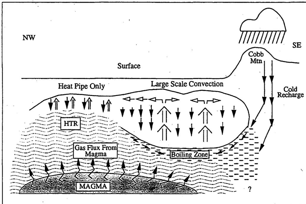
Figure 8. Schematic conceptual model of The Geysers geothermal system showing flow of steam (open arrows) and liquid (condensate and recharge water; solid arrows). HTR denotes the high-temperature reservoir.
