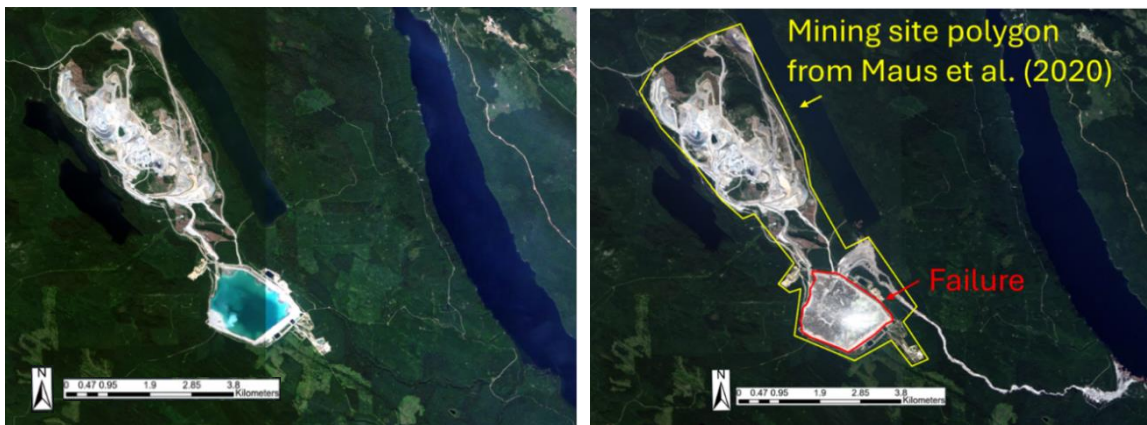
Figure 6.8: Mount Polley mine tailings dam failure, Planet© Imagery
