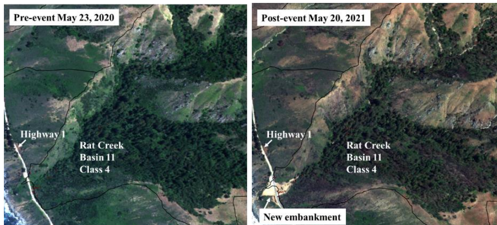
Figure 5.3: WorldView© Imagery at Rat Creek on May 2020 and May 2021 (WorldView© 2021, DigitalGlobe, Inc., a Maxar company). The imagery from May 2021 illustrates the new embankment that was placed following the washout of the previous event. The debris flow in that location is not easily discernible along its length as it is obstructed by forest vegetation
