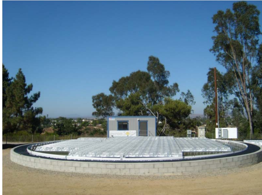
Figure 3.4 Pyron Solar's Water-Borne CPV Prototype at SDG&E Test Site (Photo courtesy of Pyron Solar)
