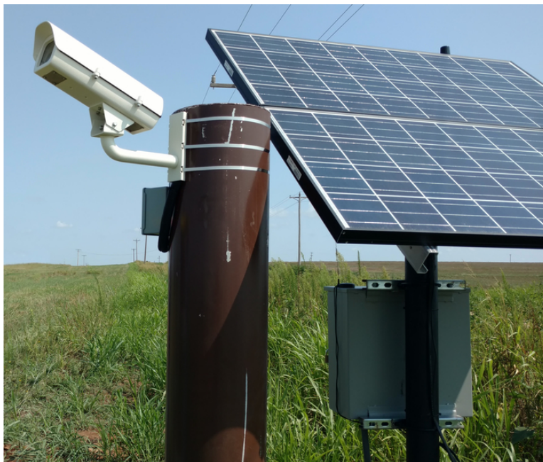
FIG. 4. One of the six cameras that comprise the stereo ring. The pole-mounted camera, tilted approximately 18^\circ from the ground, is powered by two solar photovoltaic panels connected to a lead-acid battery, and communicates with the ARM servers using a cellular network.
