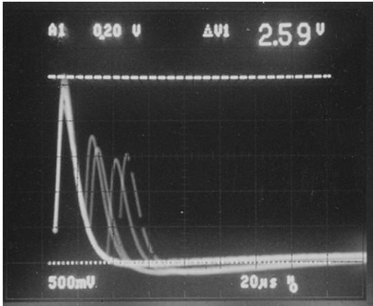
Fig. 19. Photograph of oscilloscope traces of pulses seen in LAr with 2500 ppm Kr and 1400 V applied to the drift electrode at  $\sim 1.3$  atmospheres pressure (5 psig). First (and largest) pulse is about 2.6 V, and the pulse width of  $\sim 10 \mu\text{s}$  fwhm is determined by the amplifier time constants.
