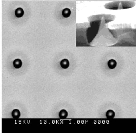
Fig. 21. Micrograph of Spindt cathode surface used in our tests. The hole diameter in the gates is  $\sim 0.75 \mu\text{m}$ . Inset: cross section through a single cathode showing the metal tip, encircled by a metal gate film and  $\text{SiO}_2$  insulator fabricated on a silicon substrate (Courtesy, Dr. Capp Spindt, SRI [29])
