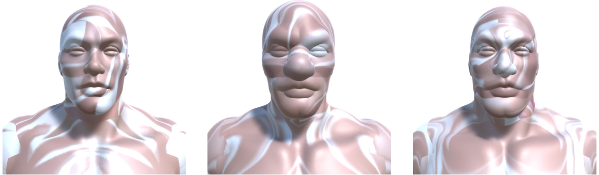
(a) Frequency 1.0, scale 0.25; flow map settings: octave 1, frequency 3, lacunarity 2, persistence 0.5 (b) Frequency 2.6, scale 0.25; flow map settings: octave 1, frequency 6, lacunarity 2, persistence 0.5 (c) Frequency 3.0, scale 0.25; flow map settings: octave 1, frequency 9, lacunarity 2, persistence 0.5
