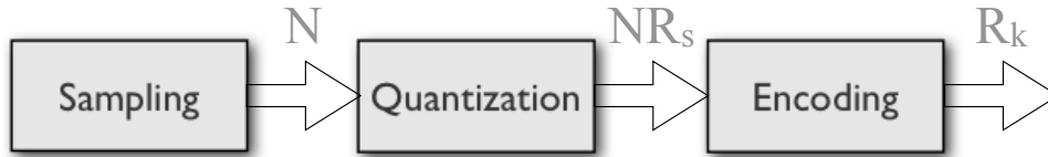
Figure 5.3: The three step digitization process. The encoding block manages the output bit-rate from the system.
