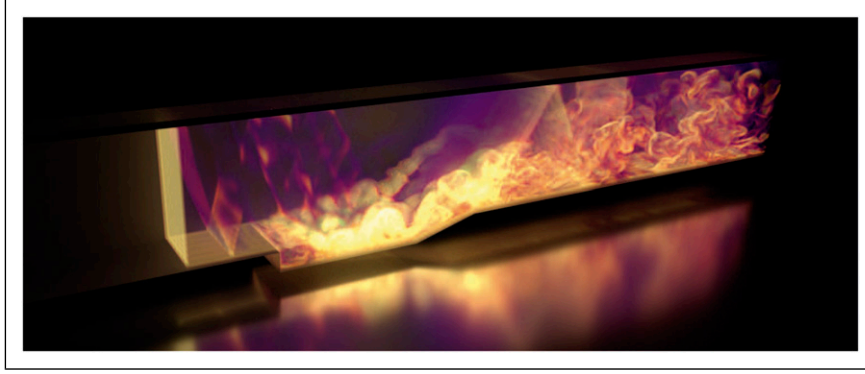
Figure 1. Simulation of direct fuel injection in a supersonic cavity flame-holder using PeleC (Sitaraman et al., 2021a,b).
