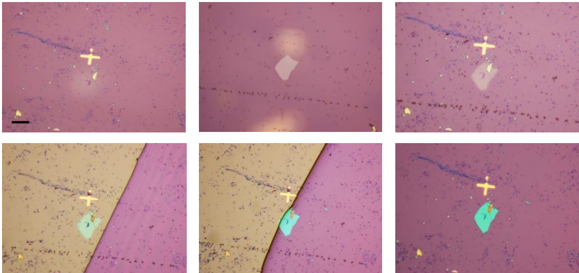
Figure 3.6: Optical images of the steps, while transferring h-BN on 1T-TaS 2 crystal. The first image is showing a dark purple flake of 1T-TaS 2 and the last image shows the green layer of h-BN covered the 1T-TaS 2 crystal. The areas with almost yellow color in the second-row images, show the PDMS layer starting to flow through the substrate. The scale bar represents 39 \mu\text{m} .
