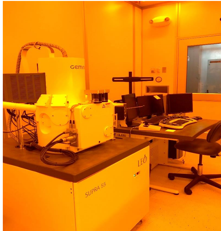
Figure 3.8: The e-beam lithography system (Zeiss Supra 55) in our clean room facility.
