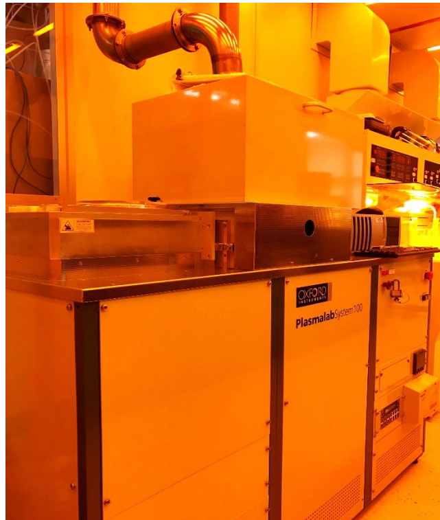
Figure 3.15: The ICP etch system (Oxford Instruments Plasmalab System 100) located in our clean rom facility.
