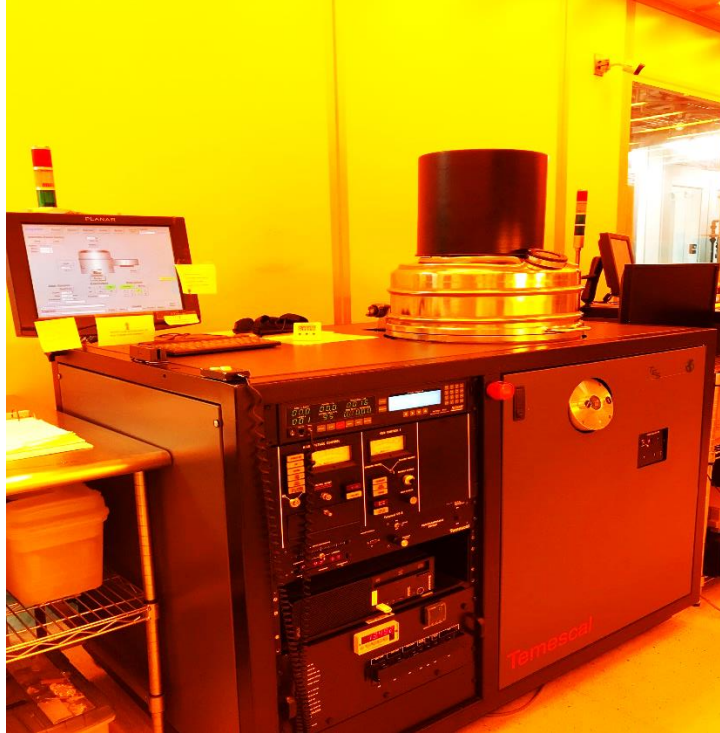
Figure 3.10: The e-beam evaporator (Temescal BJD) instrument in our clean room facility.
