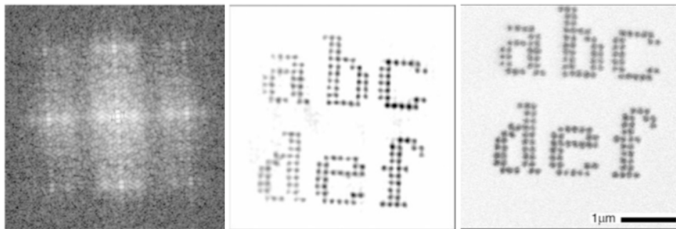
Figure 2.2: First demonstration of single-shot CDI with x-rays. the recorded diffraction pattern in logarithmic scale (left), reconstructed object (center), and SEM image for reference (right). Reproduced from [37] with permission.
