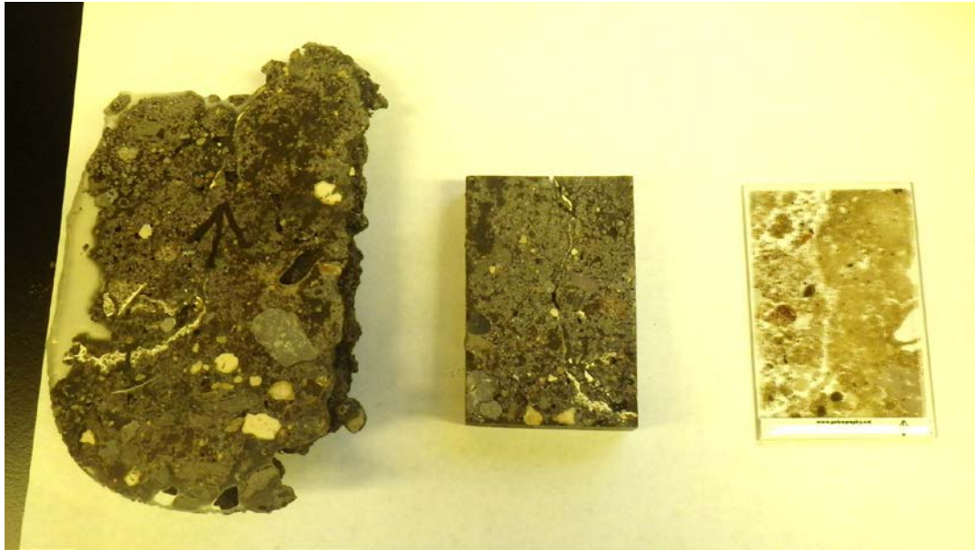
Figure 3.2: Photograph showing sequence from epoxy-impregnated block (left), to trimmed block (center), to thin section slide (right).
