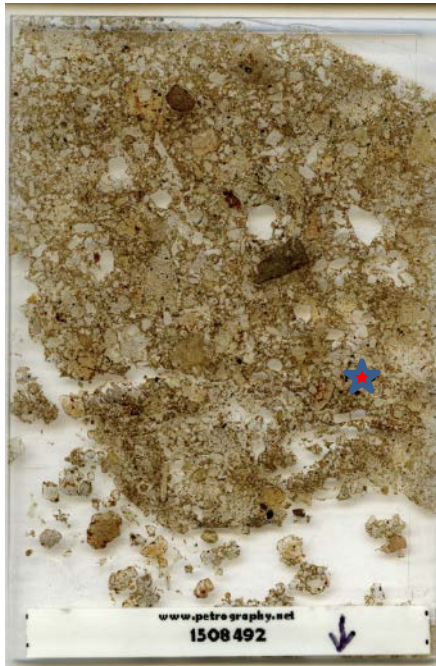
Figure 6.38: A flatbed scale of the thin section from SMS Sample 1508492 and a close up showing the organic-rich matrix. No discrete beds were identified within this sample. Scale bar is equal to 400 \mu\text{m} .
