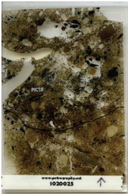
Figure 6.125: Flatbed scan of SMS Sample 1020025 and a closeup (magnification at 6.7X) in reflected light showing metal (steely blue fragments in image to right). Upper bed is Bed 1. Lower Bed is Bed 2.
