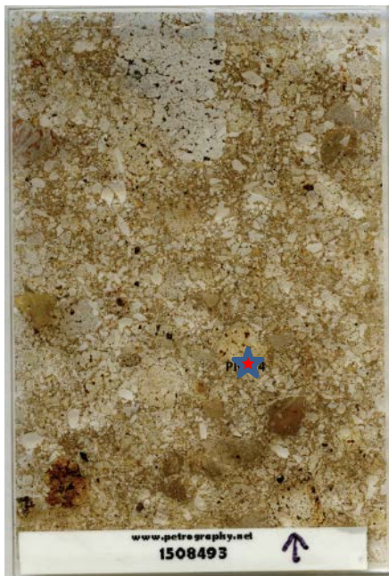
Figure 6.39: A flatbed scan of the thin section from SMS Sample 1508493 and a close up showing the sedimentary matrix. No discrete beds were identified within this slide. Scale bar is equal to 400 \mu\text{m} .
