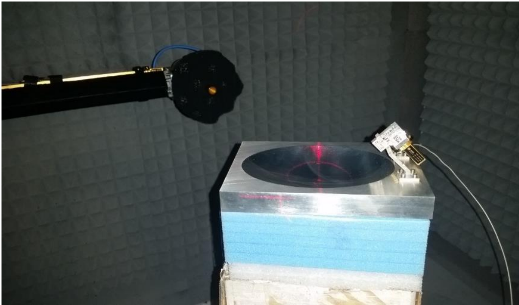
Figure 3.30 The measurement setup for the fabricated prototype of the feed reflector antenna at MVG spherical near-field chamber.
