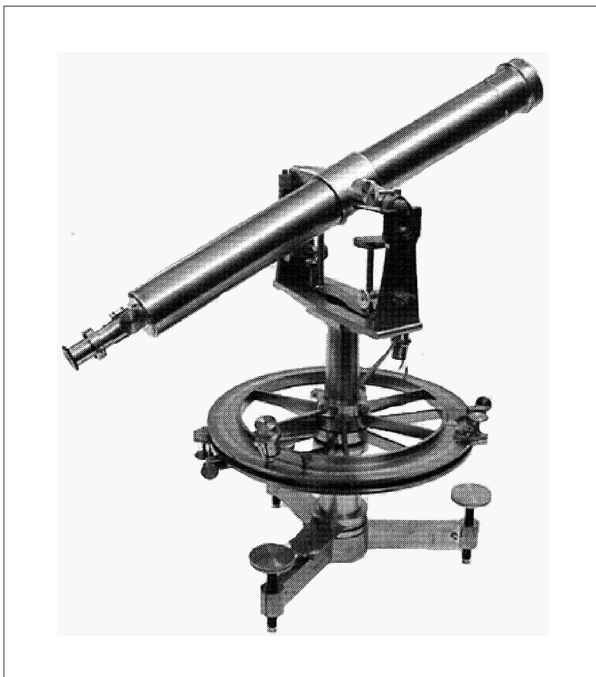
Figure 1 Theodolite typical of those used by the US Coast Survey in the 1860s. (Courtesy of NOAA Central Library.)
