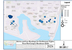
Figure 3. Lights with values higher than 4000K are problematic due to impact on circadian rhythm. Lights with lux (brightness) values that overlap with a neighbor light are problematic as that indicates excessive light intensity.
