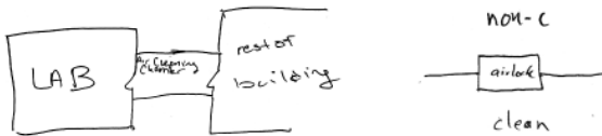
Figure 3 A multiple-space diagram of a redundant-door solution (left) and a single-space diagram (right).
