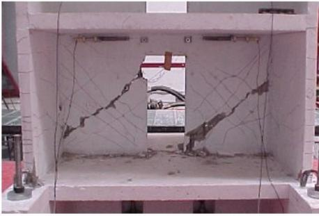
(a) Shear Failure in the First Story
