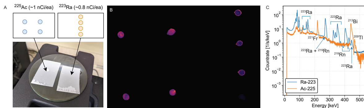
Figure 8.13: Droplet experiment setup with ^{225}\text{Ac} and ^{223}\text{Ra} . (A) Two ZnS swatches are prepared with four droplets each at approx. 1 nCi per droplet. Spatial separation provides ground truth. (B) Unprocessed iQID image of both isotopes. One ^{223}\text{Ra} droplet appears not to have been completely pipetted. (C) Energy spectra for (other samples of) equilibrium ^{225}\text{Ac} and ^{223}\text{Ra} as measured by the HPGe IDM, with select peaks annotated.
