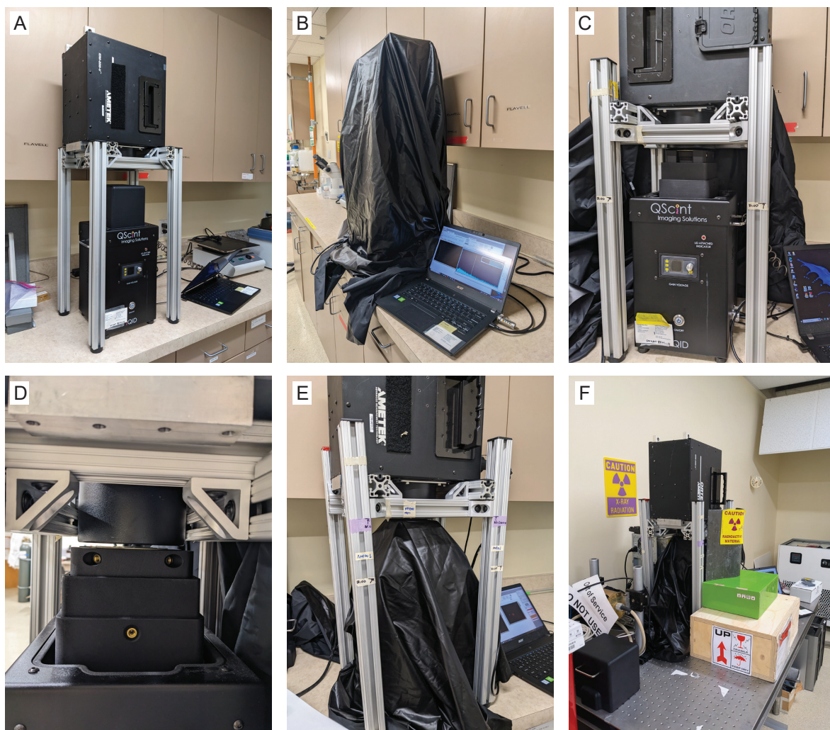
Figure 8.8: Evolution of physical system design for hybrid iQID-HPGe detection. The basic geometry stayed consistent, with the HPGc IDM supported in a detector-down orientation above the iQID sample stage as in the initial setup, (A). (B) Light-tight tarp wrapped around the setup allows iQID to be operated without the cover. (C) Inside view of (B). Adjustment of the stand brings the IDM closer to the iQID stage. (D) Close-up view of (C) showing the proximity of the HPGc head to the sample. (E) Alternative tarp placement allowing for manipulation of a sealed source on top of it. (F) Relocation of the setup to a lower-background environment with lead shielding from one direction.
