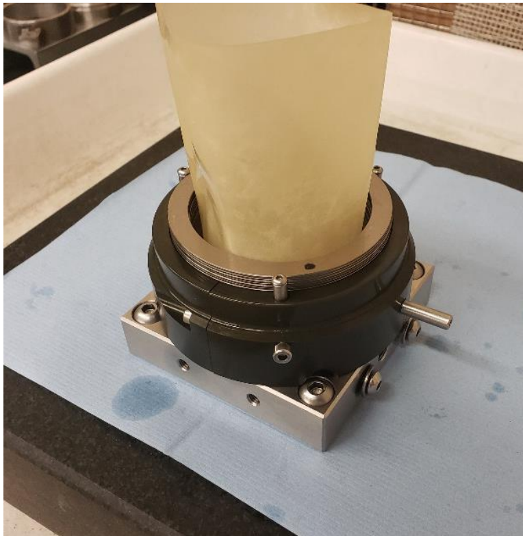
Figure A.14. Vacuum former with extension bars raised to cover all the rings.
