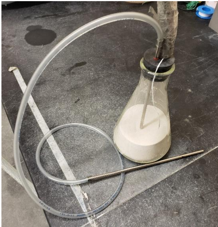
Figure A.4. Flask and tubing for vacuuming excess of soil after pluviation.
