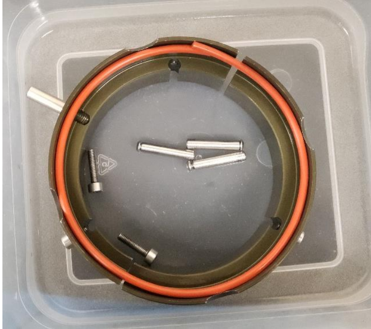
Figure A.3. Vacuum former with 3 extension bars and 1 red sealing O-ring.
