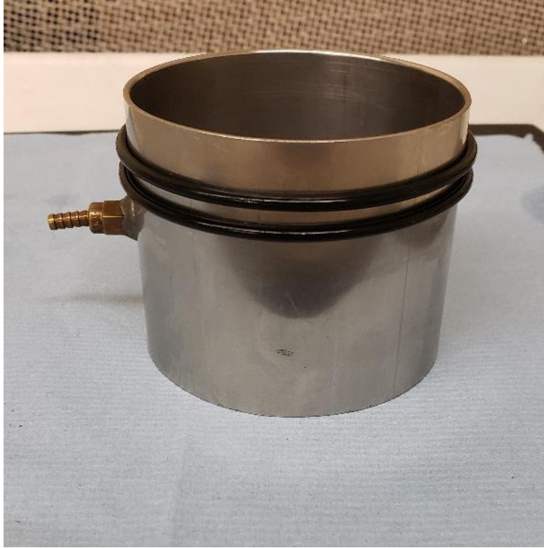
Figure A.7. O-Rings after being stretched over the expander.
