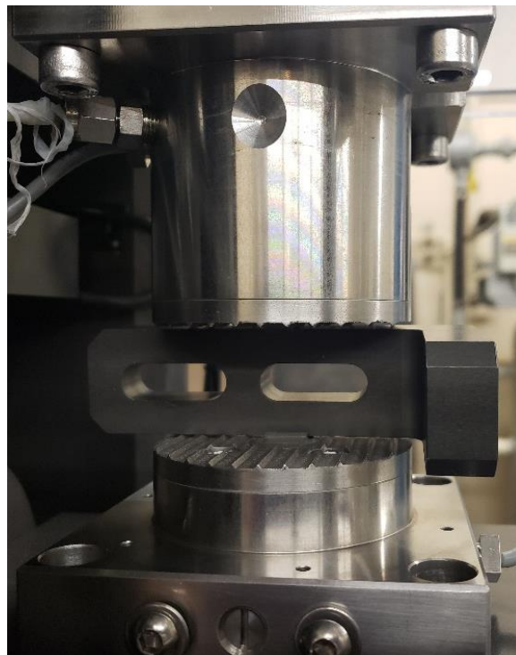
Figure A.30. Angle bracket placed between top cap and base pedestal to setup height reference.
