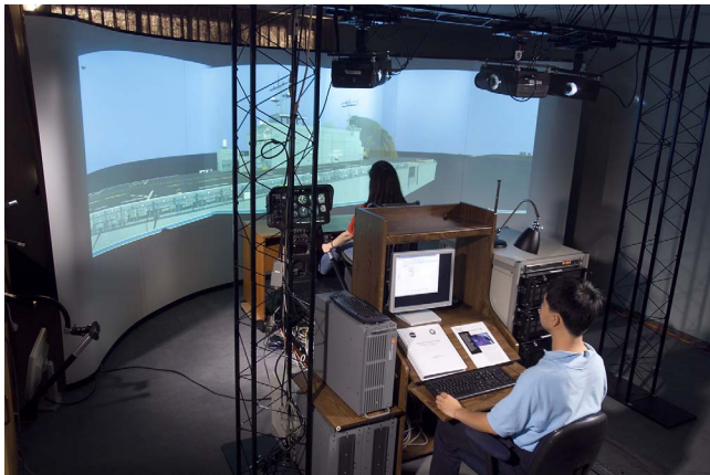
Figure 8. ART flight simulator with pilot in front of projection screen and operator at rear console
