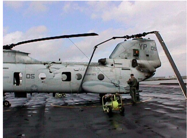
Figure 3. H-46 tunnel strike (US Govt. image, courtesy of K. Long)
