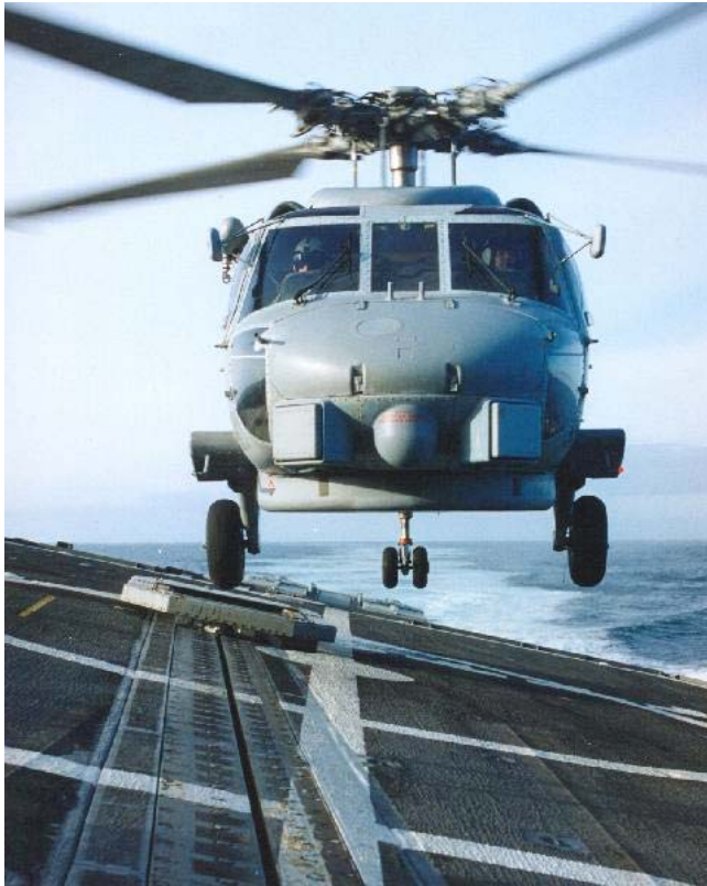
Figure 2. Helicopters landing on shipboard have to contend with high levels of pitch and roll (US Govt. image, courtesy of K. Long)
