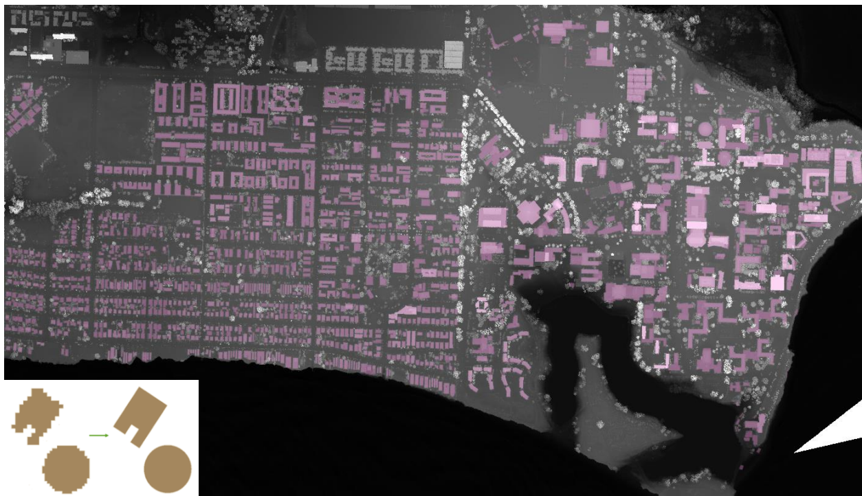
Figure 13: The building footprint after the cleaning process and manual correction.
