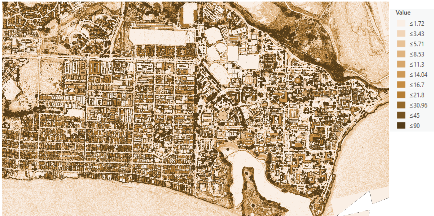
Figure 16: The slope raster of the study area is created by the Surface Parameters Tool using DEM as input.
