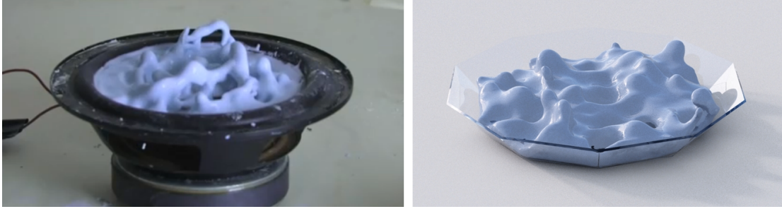
Figure 5.4: Comparison between the real [You08] and the animated shear thickening fluid in the context of the vibration experiment.
