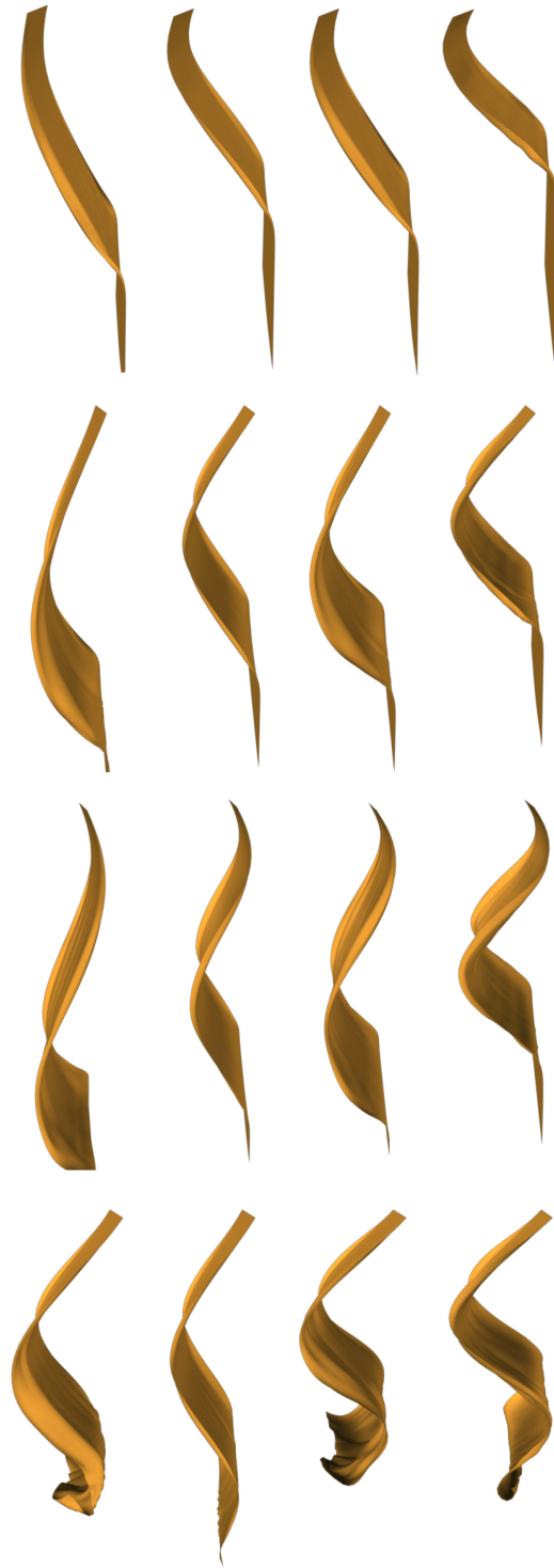
Figure 3.12: Comparisons between regular cloth deformation models using various drag models (left three columns) and fractional cloths (right-most column).
