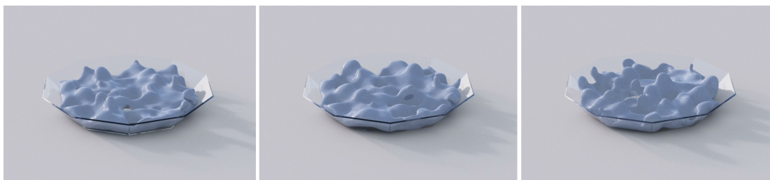
Figure 5.3: The snapshots from the vibration experiment show finger-like formations with various shapes.
