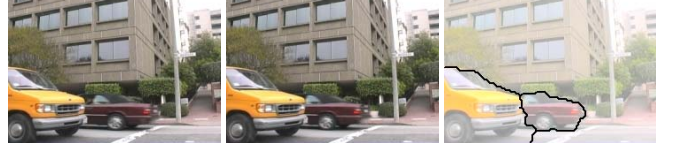
Figure 10. Motion segmentation with static camera and two moving cars. I_1 (left), I_2 (middle), segmentation (right).
