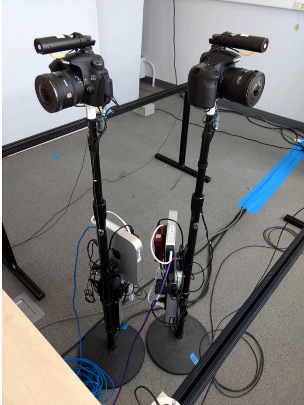
Figure 8. High-dynamic-range luminance mapping apparatus for glare measurements.
